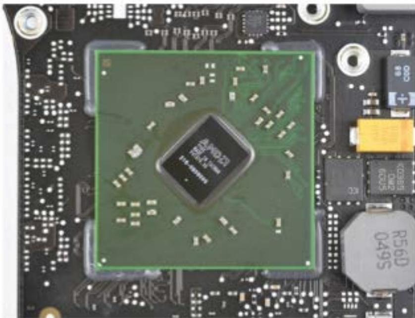
32.2 There are two layers of solder used to connect the discrete AMD GPU (referred to as the “die” below) to the logic board. The first layer consists of solder “bumps” used to connect the discrete GPU integrated circuit to the chip carrier (referred to as the “substrate” below). A second layer of solder balls connects the chip carrier to the logic board in a “ball-grid array”, as shown below:
